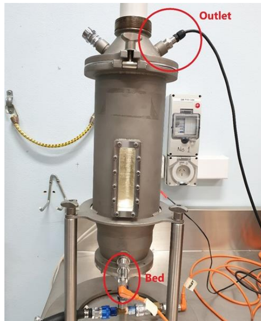
Figure 9: MBG biocatalyst yeast being prepared in a Fluidized bed dryer
